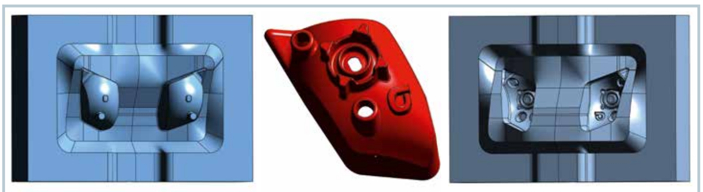
Fig. 1. Fixed (left) and moving (right) half of a two-cavity mold for headlamp reflectors of BMC (© Sigma Engineering)
