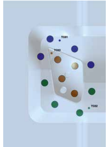
Fig. 8. Four heating cartridges each in three control circuits with the associated control points (TC01, TC02 and TC03) – this what the final layout looks like (© Sigma Engineering)
